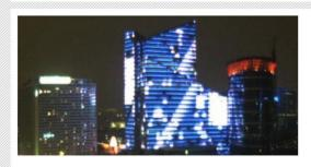
an impressive interactive full-building facade on a 145m high tower in Brussels (Dexia Tower, Belgium), on which 4200 windows can be individually illuminated by RGB-colored LED bars.
